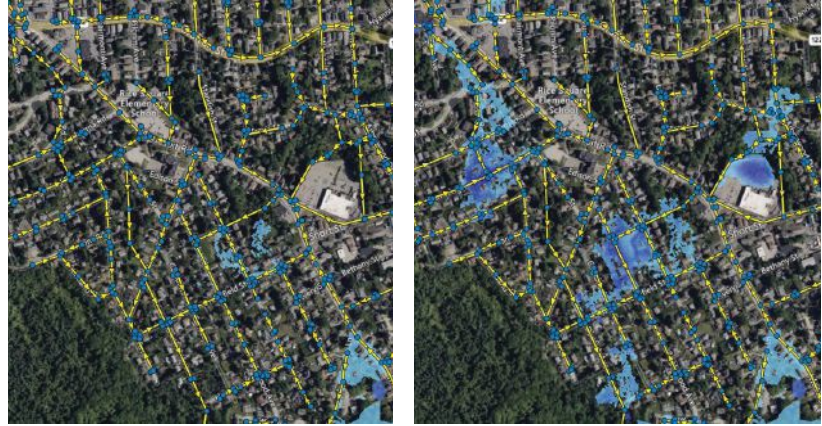
Figure 2: Example of model output comparing present and future flooding during a 10-year, 24-hour storm event.
