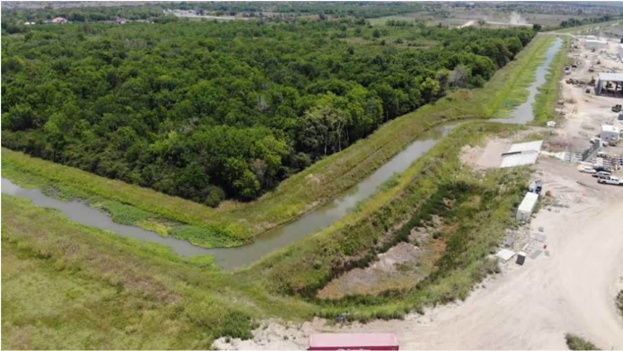
Aerial View of the Canal with Raw Water Intake lift Station in the background. GCWA plans to install a gate or gates in the west (near) end and one at the east (far) end within the channel.
