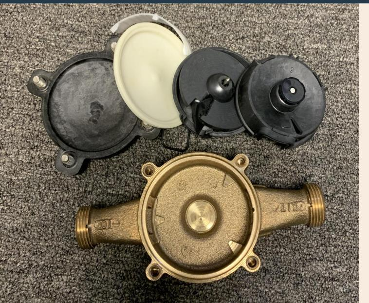
**Old**-style **meters measured water** by passing over a **disc that rotates** and turns gears.
