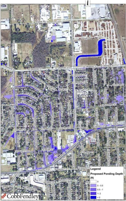
**Note\*** The proposed ponding depth exhibit (below) includes City detention (not shown) needed to provide the proposed results. Proposed detention will be included on future exhibits once location has been determined.
