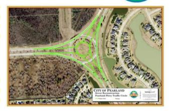
diameter by constructing a roundabout per Federal Highway Administration (FHWA) roundabout design criteria will provide the traffic calming effect needed to improve intersection safety.
