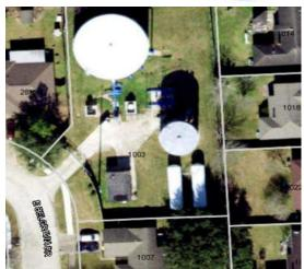
tank it leaves the site with a single 500K-gallon tank to meet the current demand of nearly 1 million gallons per day. With a peaking factor of 2.0, the peak hourly demand for the service area is approximately 1.8 MGD (1,250 gpm). As a result, the well pump can run nearly continuously to maintain water availability during these peak demands. Confirmation is based on the review of SCADA data for the Southdown WP GST Operational Levels for 2018.
