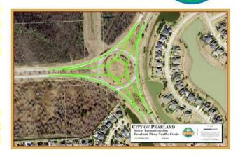
diameter by constructing a roundabout per Federal Highway Administration (FHWA) roundabout design criteria will provide the traffic calming effect needed to improve intersection safety.
