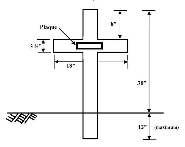
Vertical and horizontal members may be only of 2" X 4" construction. The use of concrete footings should not be allowed.
